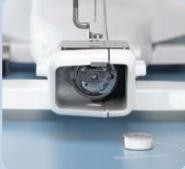
Large "M" Class Bobbin Enjoy less bobbin changes with the largest bobbins available in quilting. The Jewel also includes a high-speed rotary hook and an electric bobbin winder with variable speeds.
